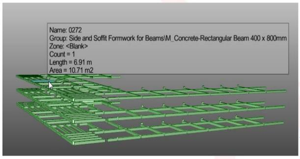
Beam Side and Soffit Formwork derived from Beam Width, Beam Height, Slab thickness and Cut length dimensions in CostX ®
