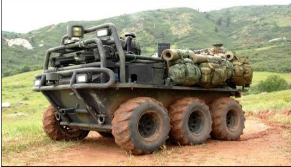
MULE ( Multi-Role-Logistics) Vehicle – Evaluated, but needs urgently a follow me WINGMAN capability – US Army
