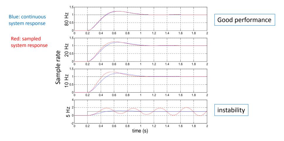
As sample rate falls performance degrades – dynamics of plant dictate sample rate and ultimately speed of controller iteration
