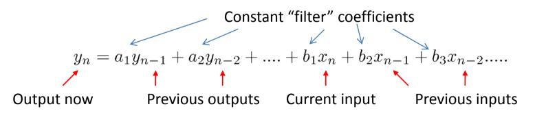
At each cycle a number of multiply and accumulates have to occur Many DSP can implement the above in a single clock cycle....
