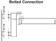
Note: Bolted connections may be requested in lieu of welded connections for an additional charge.
