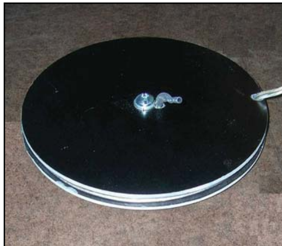
Spool Style Bifilar Antenna (above) from a Mk 2 Workstation (below)
