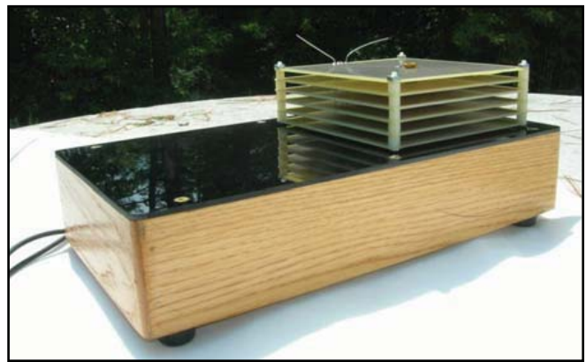
A larger enclosure allowed two arrays of antenna plates to be installed inside.
