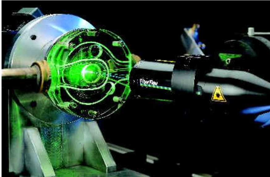
Study of the flow between rotating impeller blades of a pump
