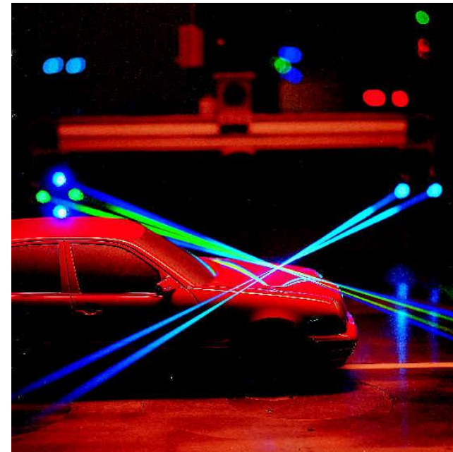
3-D LDA Measurements on a 1:5 Mercedes-Benz E-class model car in wind tunnel
