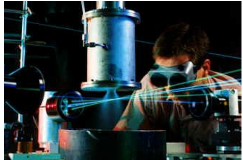
Droplet Size Distributions Measured in a Kerosene Spray Produced by a Fuel Injector
