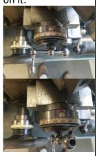
Slowly turn the cross slide handle until the tip of the lathe tool lightly touches the outside diameter of the workpiece.
