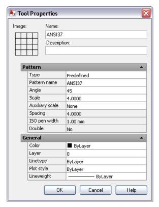
Any property that could be set in a command-line macro can be set through the tool's properties. It's an easy way to make sure the same settings are used every time.
