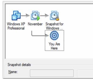
One of the most convenient aspects of using virtualization software is its support for snapshots. They allow you to preserve the current state of the virtual machine with a click of a button, and return to it with another click. VMware Workstation support multiple snapshots, which comes in very handy for “bookmarking” different stages of your analysis, so you can move back and forth during your experiments without losing important runtime details.
