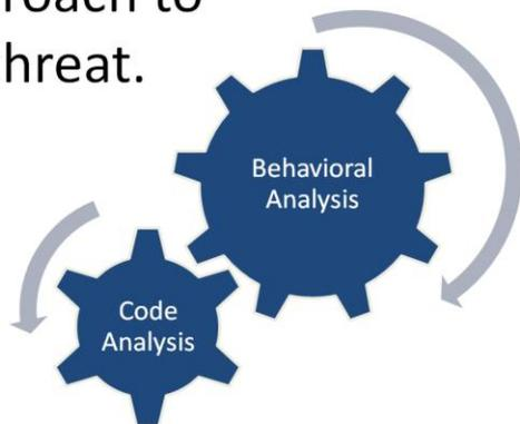
The approach to reverse-engineering that has worked for many analysts involves two key phases: behavioral analysis and code analysis. During behavioral analysis, we examine how the specimen interacts with its environment. The code analysis phase allows us to learn about the specimen's capabilities by examining the code from which the program is comprised.
