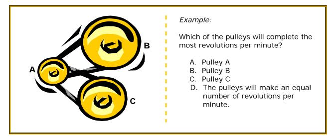
The answer is A. Notice that pulley A is the smallest of the three pulleys in the series. Because of its relative size, it has a shorter distance to travel to complete one revolution than do the larger pulleys. Thus, it can make more revolutions in the same amount of time. Another way to phrase this question would be to ask which pulley is moving fastest, in which case the same answer and supporting thought process is used.
