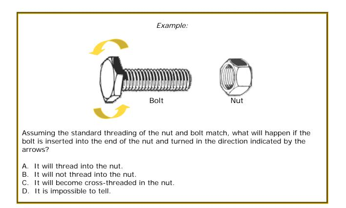
The answer is B. A bolt with standard threading will be drawn into a matching nut when turned to the right (clockwise), but will be pushed apart when turned to the left (counterclockwise). The arrows indicate that the bolt will be turned counterclockwise (left). Hence, if inserted into the end of the nut and turned, it would simply spin around and around without ever threading into the nut.
