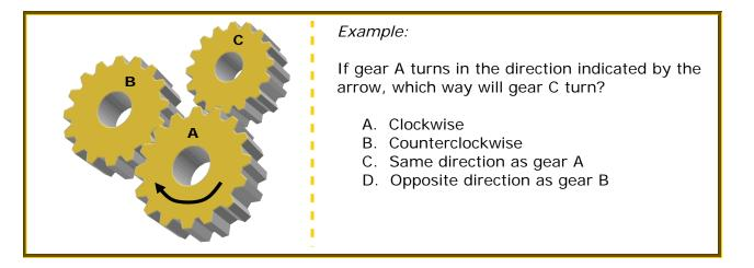
The answer is B. Notice that gear A is moving in a clockwise direction. Given the direction of rotation for gear A, we can see that the right side of the gear "tooth" on gear A is applying force to left side of the tooth on gear C. This force pushes gear C to the right, resulting in a counterclockwise rotation.
