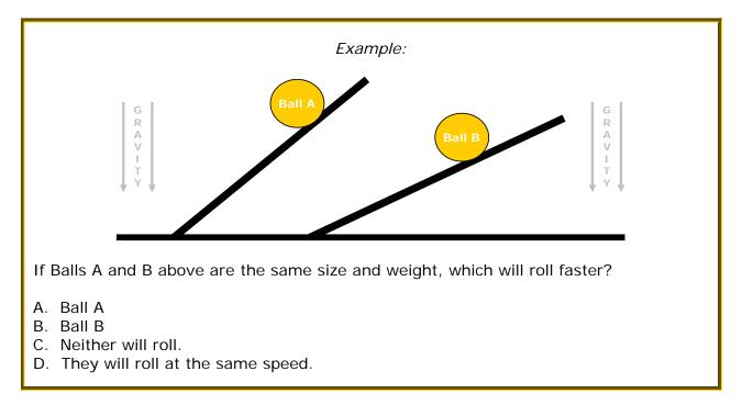
The answer is A. Because the balls are the same size, only the steepness of the incline influences how fast they will roll. As stated in the *key facts* above, the steeper the incline, the more easily an object will move downward. Hence, Ball A is able to roll faster than Ball B.
