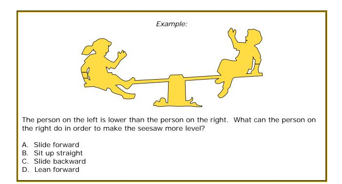
The answer is C. Because the load is nearly balanced, shifting the weight of the person on the right further away from the fulcrum will accomplish the additional work needed to balance the beam.
