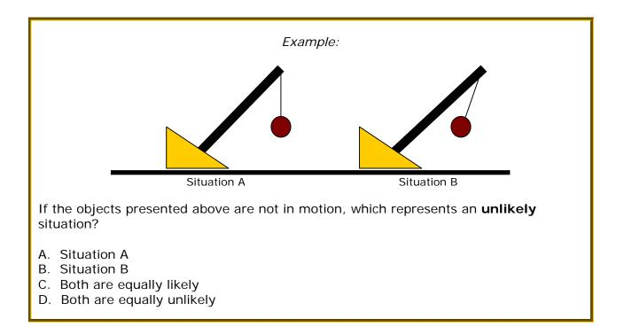
The answer is B. Because gravity always pulls objects downward, the ball at the end of the rope would be drawn straight down toward the ground. Hence, in the absence of some other force, such as a magnetic force, it is unlikely the ball would be suspended as presented in Situation B.
