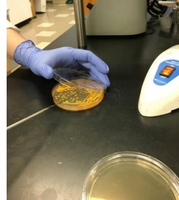
Fig. 8-Partially open the lid of the plate to gain access without exposing the plate to the open air.
