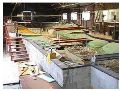
Physical models are scale representations of the same physical entities they represent. They are used primarily in engineering of largescale projects to examine a limited set of behavioral characteristics in the system. The illustration and site below are a good example of a physical model -- one of a stream and dam used to simulate the rate of outflow from the dam under a variety
