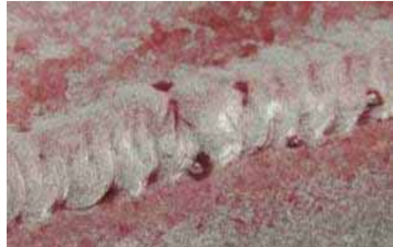
Non-relevant weld geometry indications
