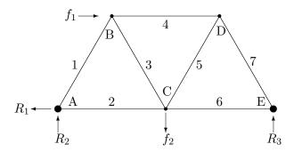
Figure 9.1: An equilateral truss. Joints or nodes are labeled alphabetically, A, B, ... and Members (edges) are labeled numerically: 1, 2, .... The forces  $f_1$  and  $f_2$  are applied loads and  $R_1$ ,  $R_2$  and  $R_3$  are reaction forces applied by the supports.
