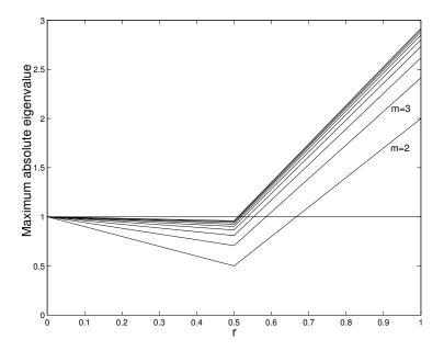
Figure 36.1: Maximum absolute eigenvalue as a function of r for the matrix A from the explicit method for the heat equation calculated for matrices A of sizes m = 2...10. Whenever the maximum absolute eigenvalue is greater than 1 the method is unstable, i.e. errors grow exponentially with each step. When using the explicit method r < 1/2 is a safe choice.
