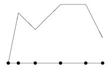
Figure 41.3: A possible finite element solution for a one dimensional object. Values are assigned at each node and a linear interpolant is used in between.
