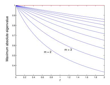
Figure 37.2: Maximum absolute eigenvalue as a function of r for the matrix  $B^{-1}$  from the implicit method for the heat equation calculated for matrices B of sizes m=2...10. Whenever the maximum absolute eigenvalue is less than 1 the method is stable, i.e. it is always stable.
