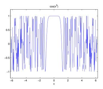
Figure 7.1: Graph of  $\cos(x^5)$  produced by the explot command. It is wrong because  $\cos u$  should oscillate smoothly between -1 and 1. The problem with the plot is that  $\cos(x^5)$  oscillates extremely rapidly, and the plot did not consider enough points.
