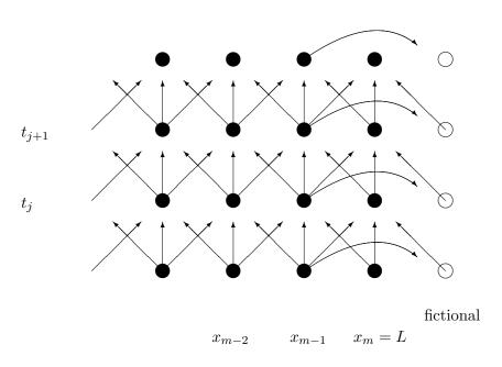
Figure 38.2: Illustration of information flow for the explicit method near the right boundary at x = L. The top figure shows a fixed boundary condition, where  $u_{m,j}$  is set to be  $g_2(t_j)$ . The bottom figure shows an insulating boundary condition. Now  $u_{m,j}$  is updated in the same way as the general  $u_{i,j}$  and an additional entry  $u_{m+1,j}$  is used with its value set by copying  $u_{m-1,j}$ .
