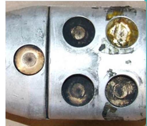
No putty in shear bolts
