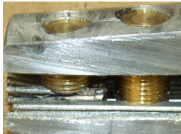
Only 1 shear bolt touching
