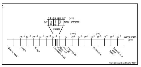
Figure 3-1: The Electromagnetic Spectrum
