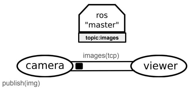
camera node sends the data to the viewer node using TCP/IP based protocol
