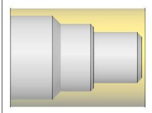
A Finishing operation along the O.D. profile will produce the desired surface finish.
