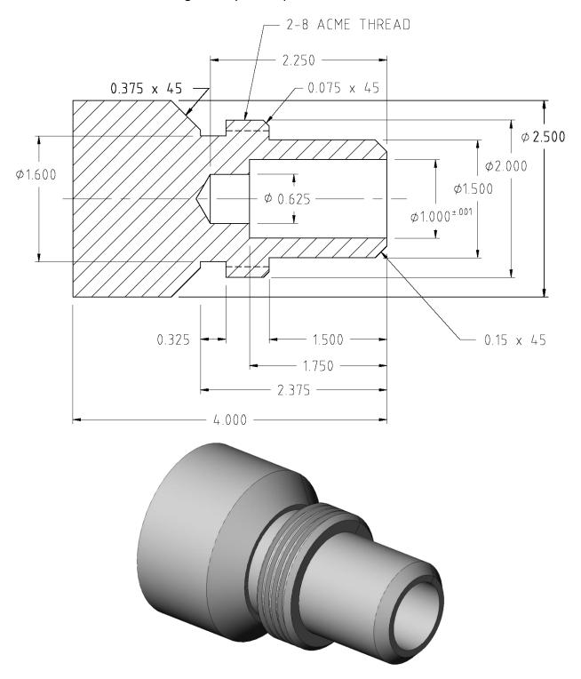
This part has many common turning features: cylindrical faces of varying diameters and lengths, chamfered edges, threads, a groove, and a hole on the center line.
