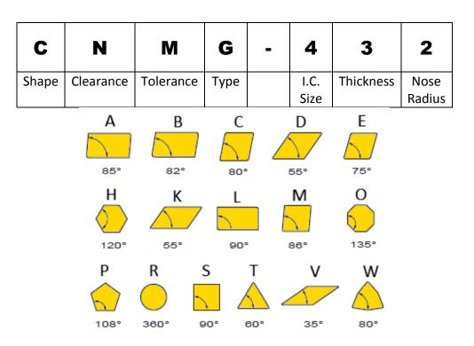
C and W type turning inserts are often used for rough machining due to their larger point angle, which makes them more rigid.
