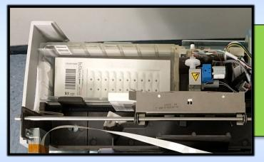
The Hydrogen Peroxide Delivery Assembly moves hydrogen peroxide solution from the Cassette Assembly to the Vaporizer Assembly. Vaporizer Assembly
