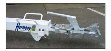
PSE 196 Embraer ERJ-175/190 Towhead Assembly (to be used on PSE-190E or PSE-190EF towbar assemblies)
