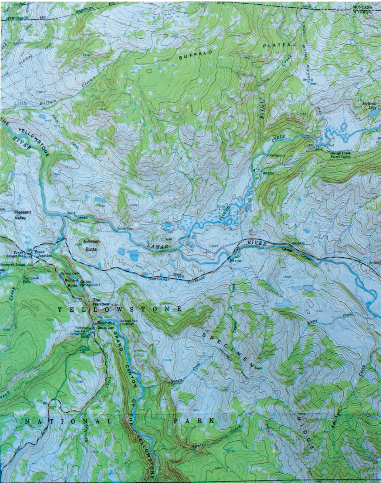
FIGURE 4 Representative section of standard topographic map: a portion of Yellowstone National Park. Note the closely spaced contours along the Grand Canyon of the Yellowstone and edges of plateaus, the shapes of contours that cross streams, the closed contours around hills (for example, Junction Butte), and the swampy flat area (along Slough Creek).
