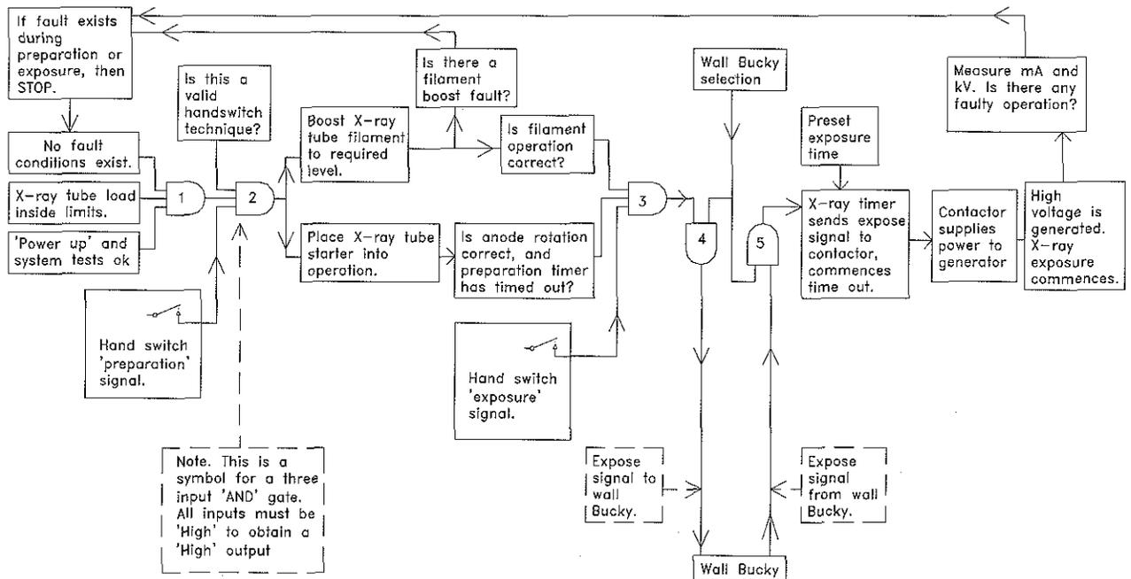
This diagram is to illustrate the basic sequence on making an X-ray exposure. In this instance, the wall Bucky has been selected prior to preparation.
