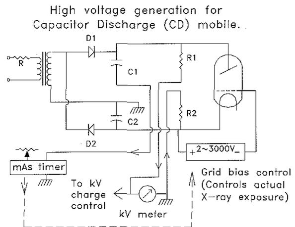
On +ve half cycles, D1 conducts, charging C1. On -ve half cycles, D2 conducts, charging C2. This continues until capacitors are charged to the required kV.
