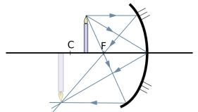
An image formed by a spherical mirror<sup>11</sup> (Available in the online resource: *Facilitator's Guide High Resolution Graphics*)
