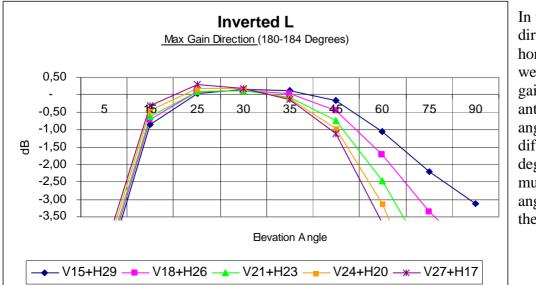
In this graph – the direction of the horizontal wire – we see a small gain of the higher antenna at low angles, no difference at 30 degrees, and a much more high angle radiation by the low antennas.
