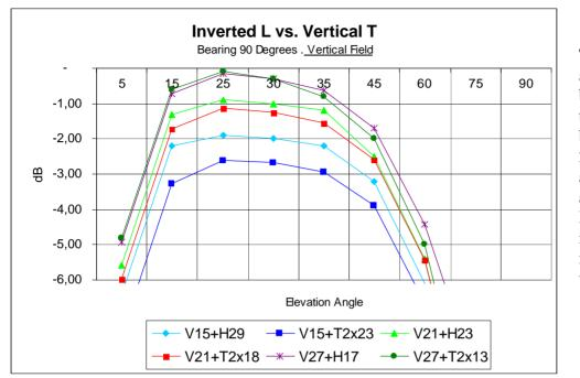
The vertical field at 90 degrees bearing is almost the same from both antennas 27m. high; there is a small difference at 21m., while lowering at 15m. it's better the inverted L than the vertical T.
