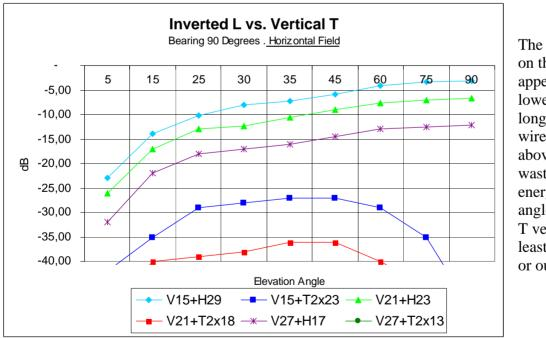
The best antenna on this graph appears to be the lowest one (with longest horizontal wire), but we saw above that it wastes too much energy on higher angles. T verticals are at least 25dB down or out of picture.
