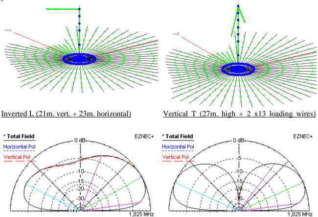
The next graph compare them with the two different Eznec ground types: Minimec with a loading resistor and real accuracy with 60 radials.
