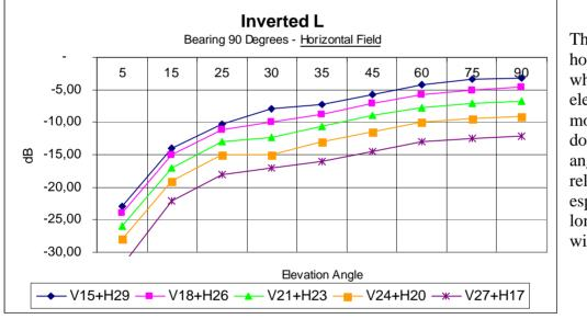
This is the horizontal field which, at low elevation angles, is more than 10 dB down, but at high angles becomes relevant, especially for the longer horizontal wire antennas.
