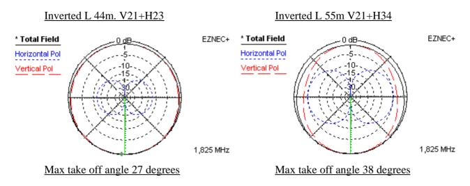
But in the following vertical plots, where the extended traces are added to the primary one, (black, which is the resonant 44m. inverted L), it seems that too much energy is wasted to warm up the sky!
