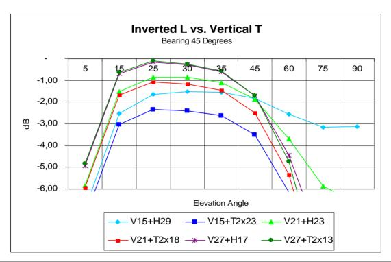
Bearing to Europe: at 27m. height there is no difference between Inverted L and Vertical T; at 21m. the inverted L seems better.
