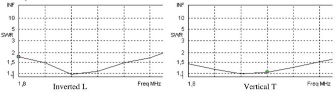
As expected, the vertical T is little broader the inverted L, but both are perfectly matched to the 50 ohms feeding line by means of easily manageable components with low losses.
