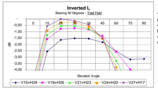
This is broadside to the horizontal wire, and the four higher antennas show about half dB better. Now let's look separately at the two field components; in the previous azimuths there was no trace of the horizontal field, but at 90 degrees – broadside to the wire – it becomes relevant.
