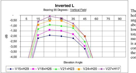
The vertical field holds up at low angles, but it's about half dB lower than the total field, meaning that there is also a small contribute from the horizontal component.
