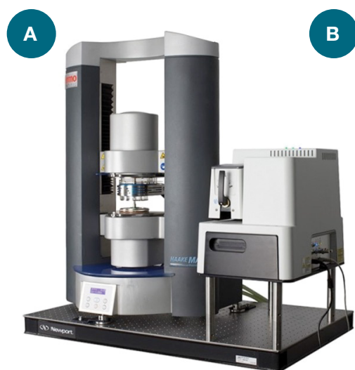
Figure 1. (a) The Thermo Scientific™ HAAKE™ MARSxR RheoRaman System. (b) Schematic diagram of the MARSxR RheoRaman system (showing side and top views of the rheometer sample stage). The iXR Raman spectrometer is free-space coupled to the MARS rheometer using lens tubes and mirrors that direct light into a 20x objective. The objective focuses the incoming laser (green dashed line) and collects the back-scattered Raman light (yellow) coming out of the sample sitting atop the rheometer stage.
