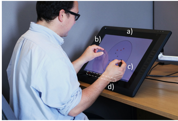
Figure 7: System setup: pen and touch display (a), user's multi-touch input (b), pen input (c), eye tracker (d).
