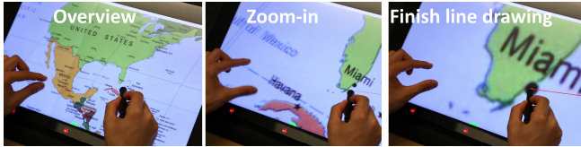
Figure 3: Pen-touch: While users are drawing a line, users can zoom into the pen’s position and then precisely finish the line drawing.
