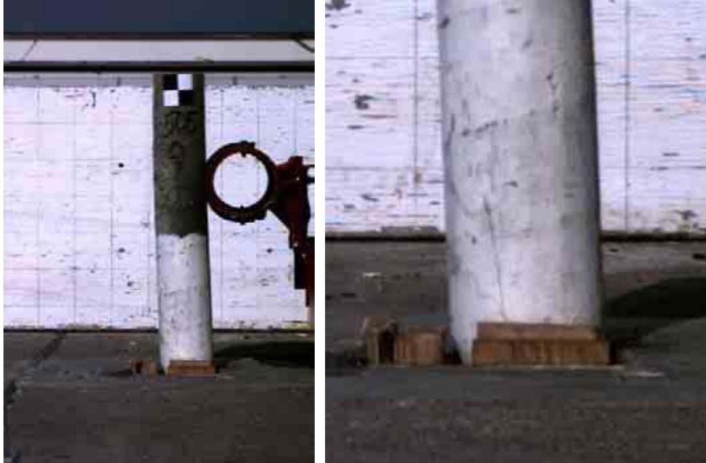
Figure 12. Post Bending Prior to Fracture - Frame 107
