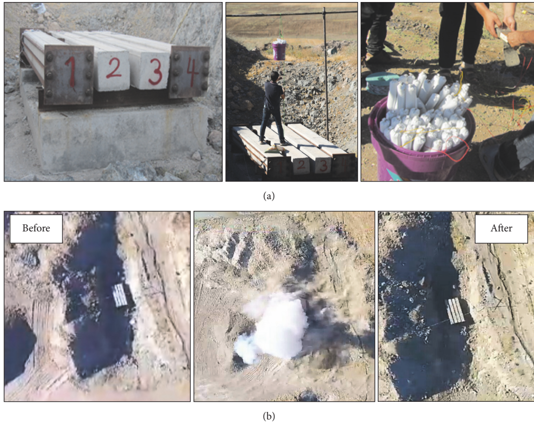
FIGURE 7: Test setup for blast loading of the specimen (a) and aerial photos of the explosion event (b).
