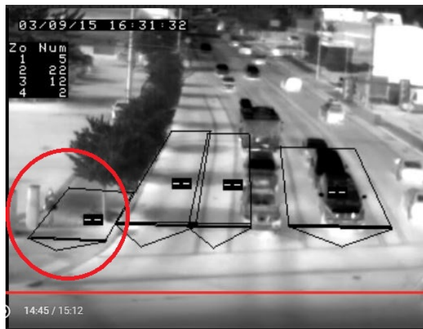
Figure 5.18: Thermal Camera False Negative – Sidewalk SB Hall & 99W
