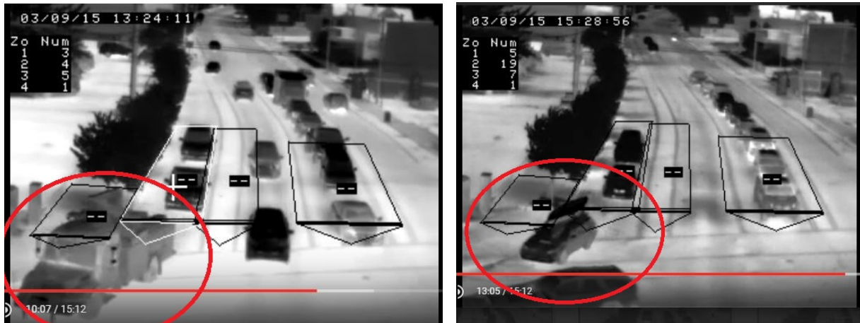
Figure 5.17: FLIR False Positives – Southbound Right Turn Lane Hall & 99W
