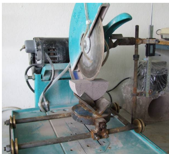
Figure 5.7 Opening of notches to SCB specimen
