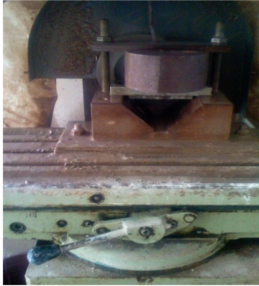
Figure 5.9 Flattening of the ends of the specimen in the grinding machine
