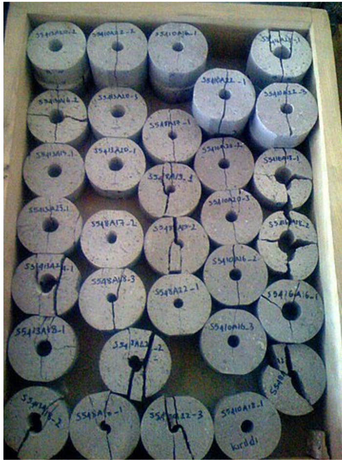
Figure B.1 Some of the 54 mm specimen photos after the experiments
