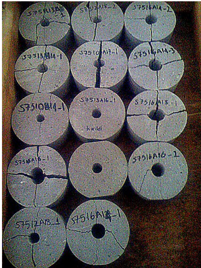
Figure B.2 Some of the 75 mm specimens after the experiments
