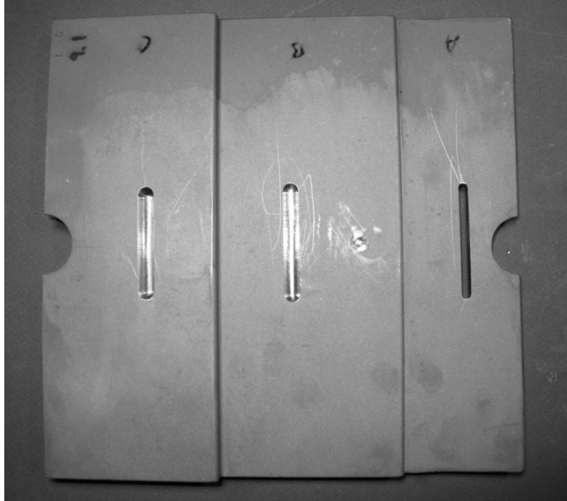
Figure 3. Staircase blank prepared with machined grooves for weld repair.
