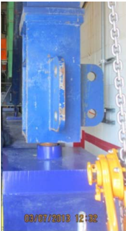
Figure 16 – Omnidirectional pin at base of column
