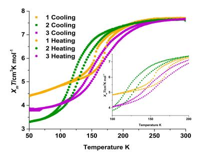
**Figure 2.** Magnetic susceptibility  $\chi_{\rm M}T$  versus T plots for 1–3, at a scan rate of 4 K/min over the temperature range of 50–300 K, in both the cooling (square) and heating (circle) modes. For clarity, the inset shows the spin transition between 100 and 200 K.
