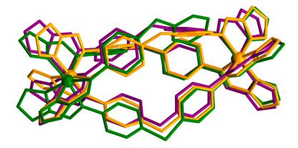
**Figure 3.** Schematic overlay representation of the X-ray structures of **1** (orange), **2** (green) and **3** (purple) at 100 K. Counter Ions, solvent molecules and hydrogen atoms have been excluded for clarity.
