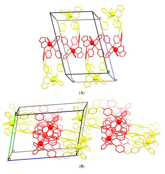
**Figure 7.** Schematic representations of the crystal packing structure of **3** at 100 K showing the packing of HS (yellow) and mixed spin state (red) Fe(II) centres in undulating rows of metal ions with similar spin states throughout the crystal lattice. Image (**A**) shows the packing in two-dimensions and image (**B**) shows three-dimensional arrangement of Fe(II) centres. Hydrogens, solvent and counter ions have been omitted for clarity.
