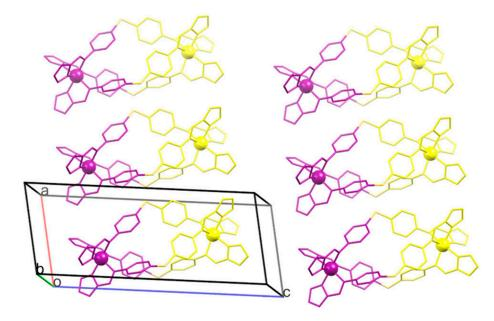
**Figure 5.** Schematic representation of the X-ray crystal structure of **2** at 100 K showing the distribution of high (yellow) and low spin (purple) Fe(II) centres along the crystallographic *c*- and *a*-axis. Hydrogens, solvent and counter ions have been excluded for clarity.
