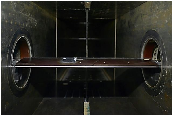
Fig. 1. The investigated airfoil in the test section of the IoA N-3 trisonic wind tunnel
