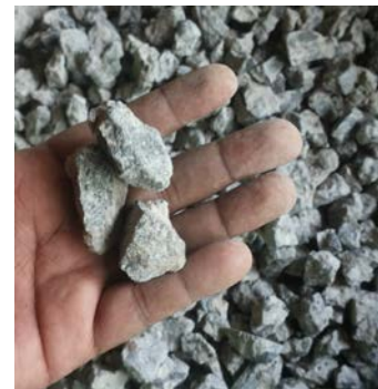
Recycled concrete aggregate
