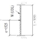
18) For column node 273 to 274 M = P x e, P = W x L, W = a x b x pressure load e = L/2 = 3.05/2 = 1.525m M = P x e, 1664.8 = P x 1.525, hence P = 1091.70 kN
