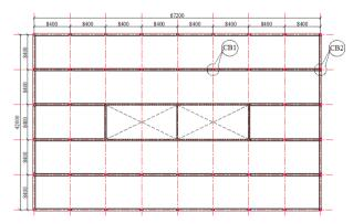
Fig.3 Typical Floor Plan (showing beams and columns)
