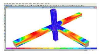
Fig.13 Connection CB2, Finite Element Model (load case 306)
