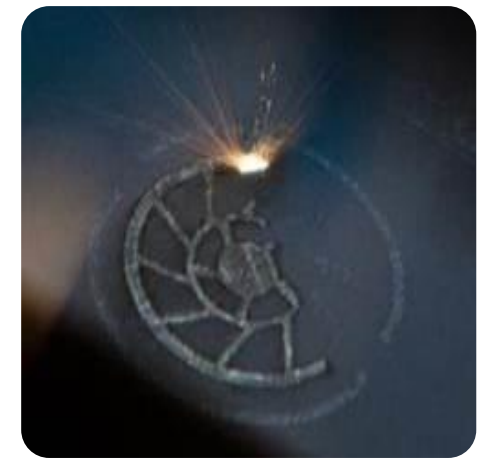
Fuel nozzle swirler prototyping
