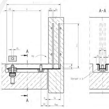
Parapet anchor, with adjustement screw, standard unit, Part no. 04BA203- Md -L
