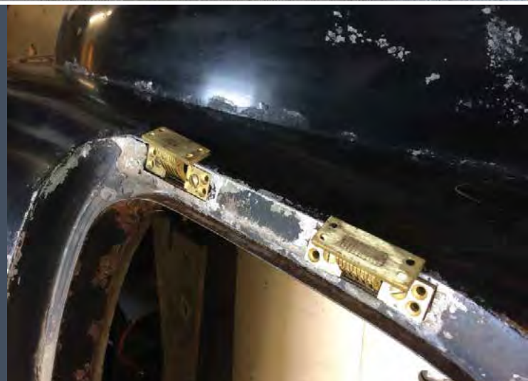
This photo shows the trunk of the car above, using the Model # 121 SOSS Hinges, which were part of the original production.
