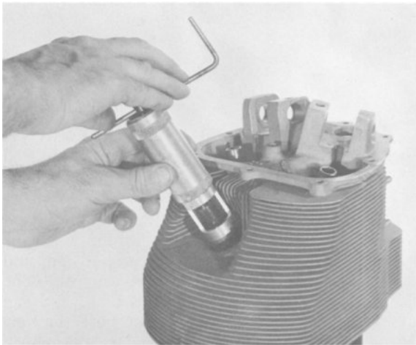
FIGURE 5-4. INSTALLING SPARK PLUG HOLE HELICAL INSERT.
