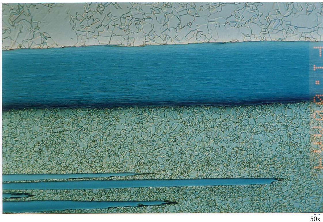
Figure 53: Superconductor CuSn+NbTi+Ta with Cu Layer after Ion Beam Etching (Specimen 2, longitudinal), Overview Micrograph with DIC, Parameter: multiple etching, please see above.
