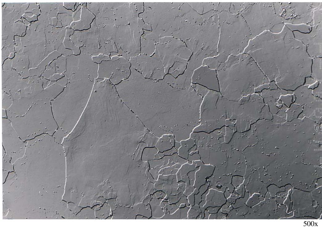
Figure 11: Texture of the Ferrite Stainless Steel X7Cr13 with Carbides at the Grain Boundaries, (Specimen A/3), Ion Beam Etched, Parameter: 6 kV / 405 \mu A / 12 mins, 45°, Rotating
