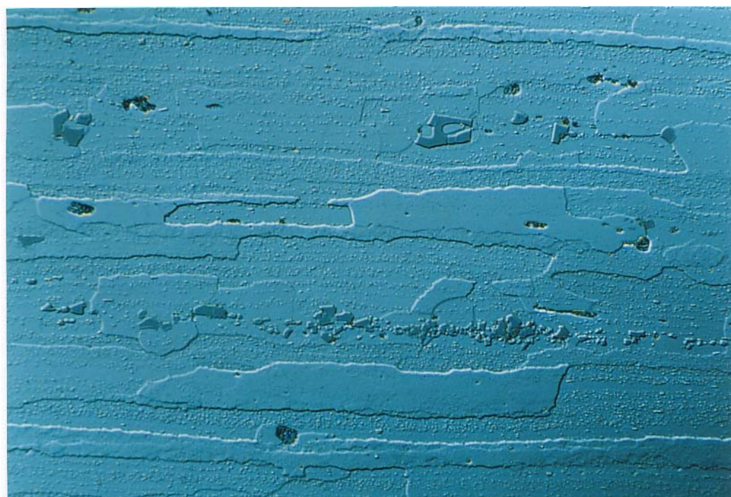
Figure 43: Texture of the Rolled Al Alloy AlMg4.5Mn/15G after Ion Beam Etching (Specimen 5), Micrograph with DIC, Grain Boundaries Developed, Grain Surfaces Rough to Grainy, Parameter: 6kV / 405 \mu A / 8mins, 55 ^\circ , rotating
