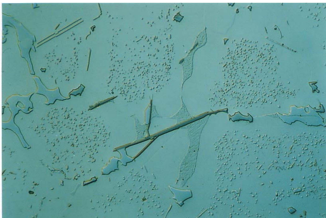
Figure 78: Soldered Joint made of the Nickel Alloys Nimonic (base material) and NB125 (solder) after Bombardment with Ar Ions (Specimen 13), Micrograph with DIC, Slight Texturing of Base Material GW, Solder Matrix and Solder Phases, Section of Figure 76, Parameter: cf. Figure 76
