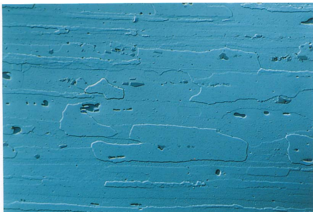
Figure 42: Texture of the Rolled Al Alloy AlMg4.5Mn/15G after Ion Beam Etching (Specimen 6), Micrograph with DIC, Grain Boundaries Developed, Grain Surfaces Relatively Smooth, Parameter: 6kV / 405 \mu A / 6.4mins, 45 ^\circ , rotating
