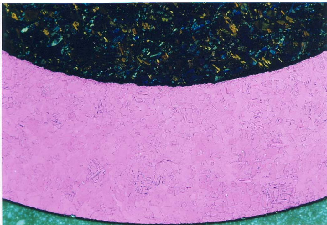
Figure 59: Partial Area of the Superconductor of Ag Mantle with Ceramic Core after Ion Bombardment (Specimen 1), Grain Boundaries and Twins of the Ag Mantle Developed, Micrograph with POL Filters, Parameter: 6 kV / 385 \mu A / 4.4 mins, 45°, rotating
