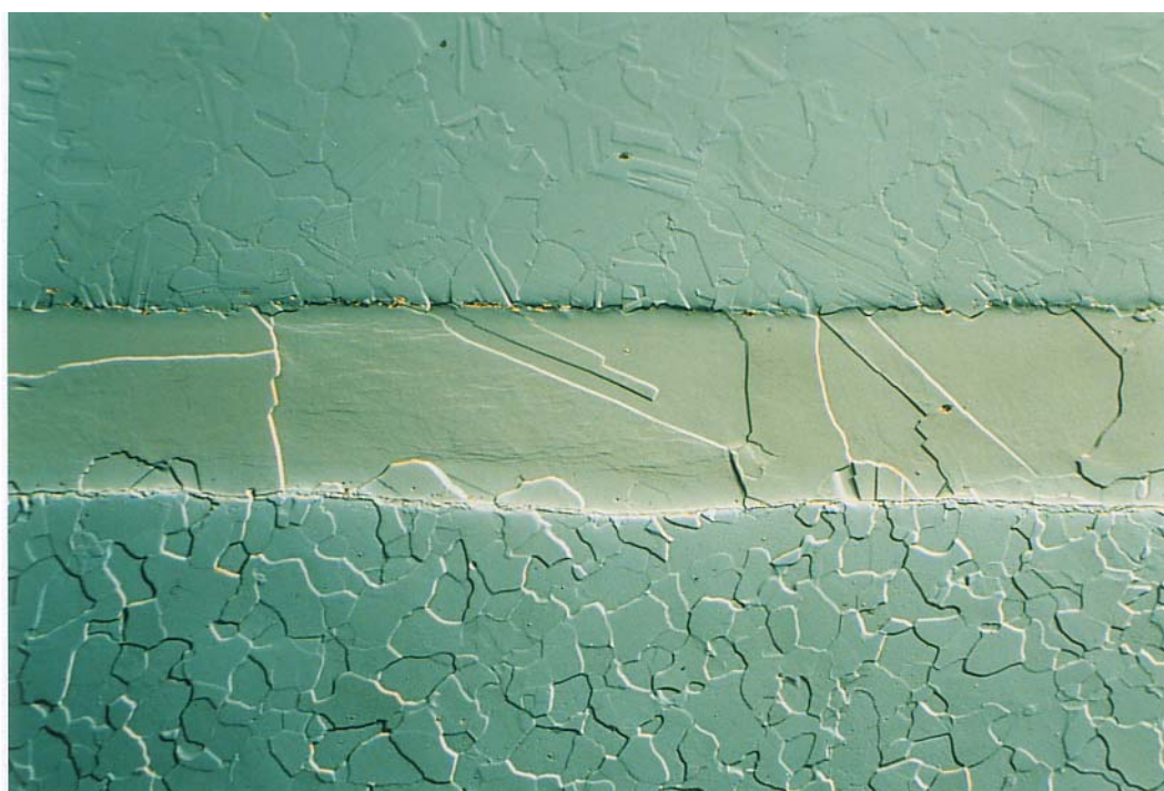
Figure 71: Weld Link of Hastalloy on Plain Steel with Ni Intermediate Layer after Bombardment with Ar Ions (Specimen 1), Micrograph with DIC, Texturing of Matrix, Welds and Ni Layer, Enlarged Section of Figure 68
