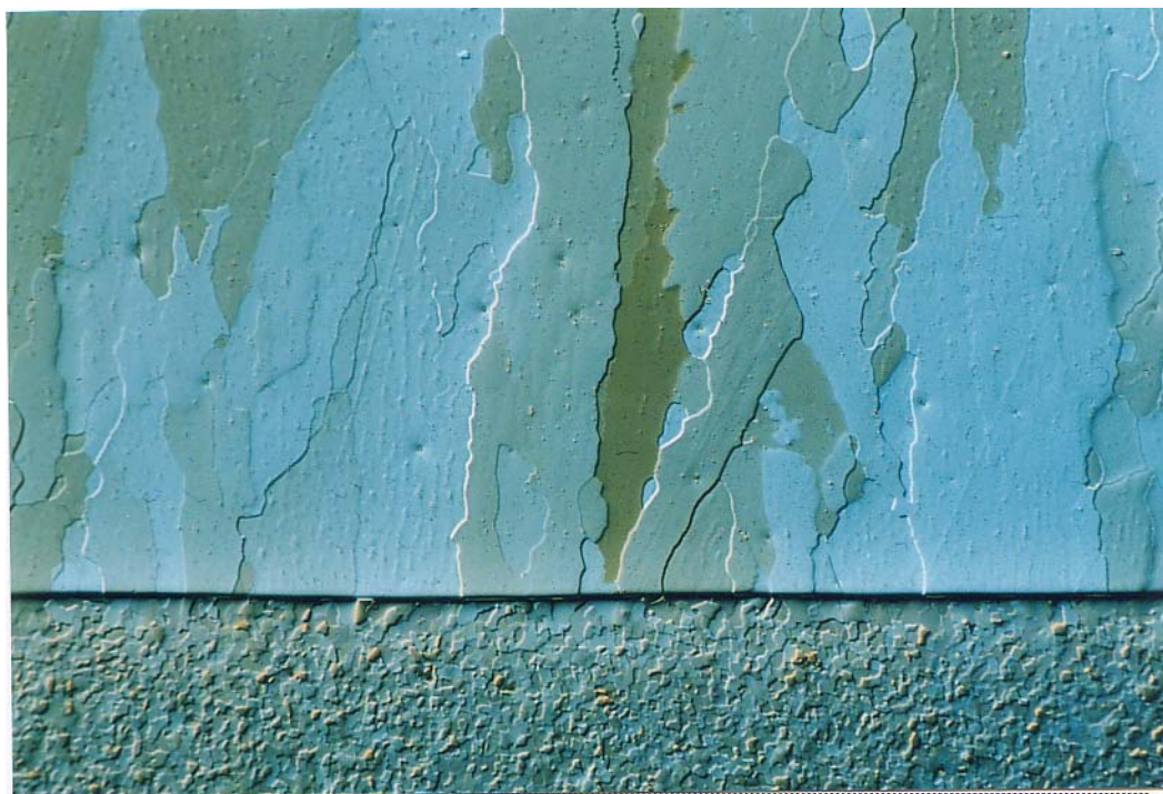
Figure 67: Build-Up Welds derived from a Ni Alloy on Boilerplate HII after Bombardment with Ar-Ions and additionally with Oxygen (large specimen), Micrograph with DIC, Same position as Figure 66, enhanced contrast by means of Tarnish Layer, Parameter: Ar Etching (please see above) + O 2 Etching (8.5 kV / 385 μA / 5.2 mins, vertical, rotating)
