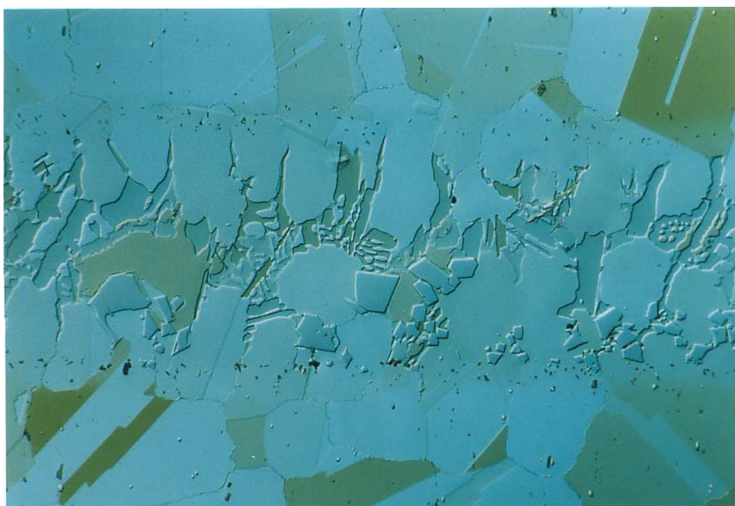
Figure 74: Soldered Joint made of the Nickel Alloys Nimonic (base material) and NB30 (solder) after Bombardment with Ar ions and additionally with Oxygen (Specimen 8F), same position as Figure 73, Enhanced contrast as a result of the tarnish layer, Parameter: Ar Etching (please see above) + O 2 Etching (8.5 kV / 445 \mu A / 3.4 mins, vertical, rotating)
