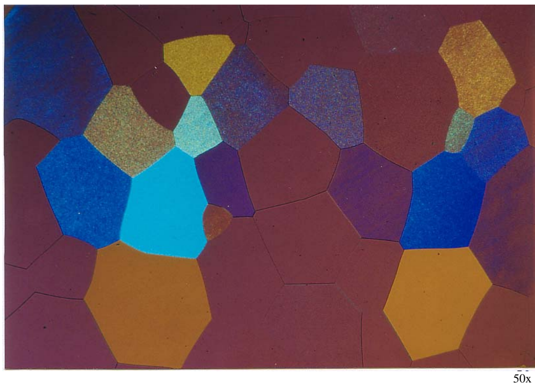
Figure 33: Structure of High-Purity-Aluminium after Ion Beam Etching (Specimen 4), POL Micrograph (sufficient rough to grainy grain surfaces appear in color), Parameter: 6 kV / 405 \mu A / 12 mins, 52,5°, rotating + 6 kV / 405 \mu A / in total 24 mins, 45°, rotating
