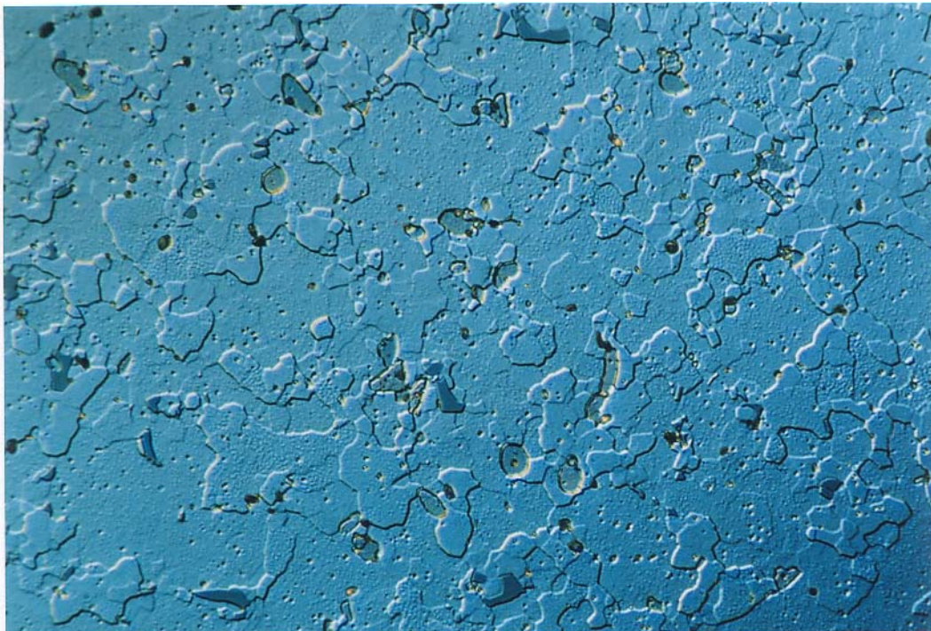
Figure 39: Structure of the Machining Alloy AlMgSiPb after Ion Beam Etching (old specimen), Micrograph of edge of the etch mark with DIC, Lead droplets are retained in addition to other intermetallic phases, Parameter: 6 kV / 400 \mu A / 8 mins, vertical and 4 kV / 120 \mu A / 8 mins, vertical
