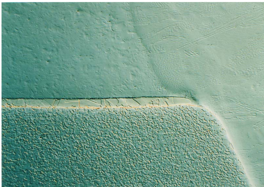
Figure 68: Overview of the Weld Link of Hastalloy on Plain Steel with Ni Intermediate Layer after Bombardment with Ar Ions (Specimen 1), Micrograph with DIC, Slight Texturing of Matrix, Welds and NI Layer,
