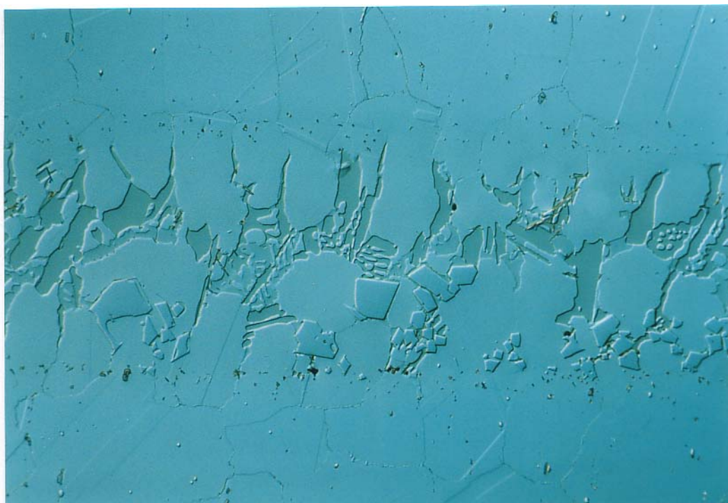
Figure 73: Soldered Joint made of the Nickel Alloys Nimonic (base material) and NB30 (solder) after bombardment with Ar ions (Specimen 8F), Micrograph with DIC, Slight Texturing of Base Material, Solder and Transition, Parameter: 6 kV / \approx 435 \mu A / in total 8.4 mins, 45°, rotating
