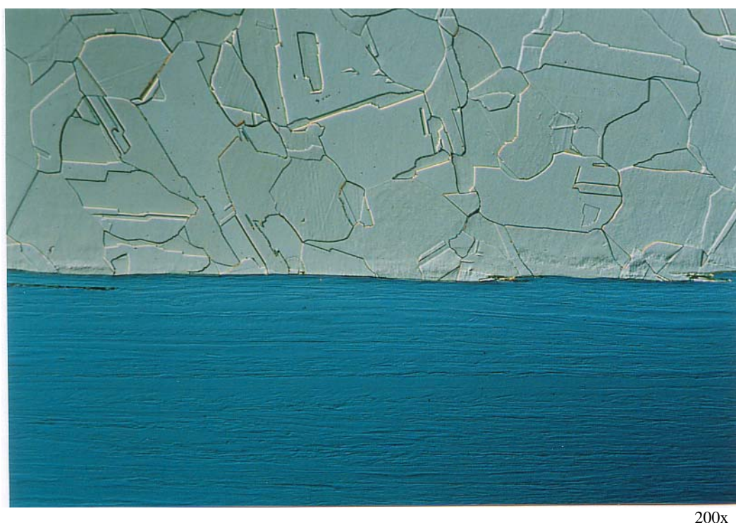
Figure 54: Superconductor CuSn+NbTi+Ta with Cu Layer after Ion Beam Etching (Specimen 2, longitudinal), Ta with Cu Coating, Section from Upper Area of Figure 53, Micrograph with DIC, Parameter: 6 kV / 405 \mu A / 12 mins, 45°, rotating + 6 kV / 405 \mu A / 2.4 mins, vertical, rotating + 6 kV / 390 \mu A / 2 mins, 10°, rotating
