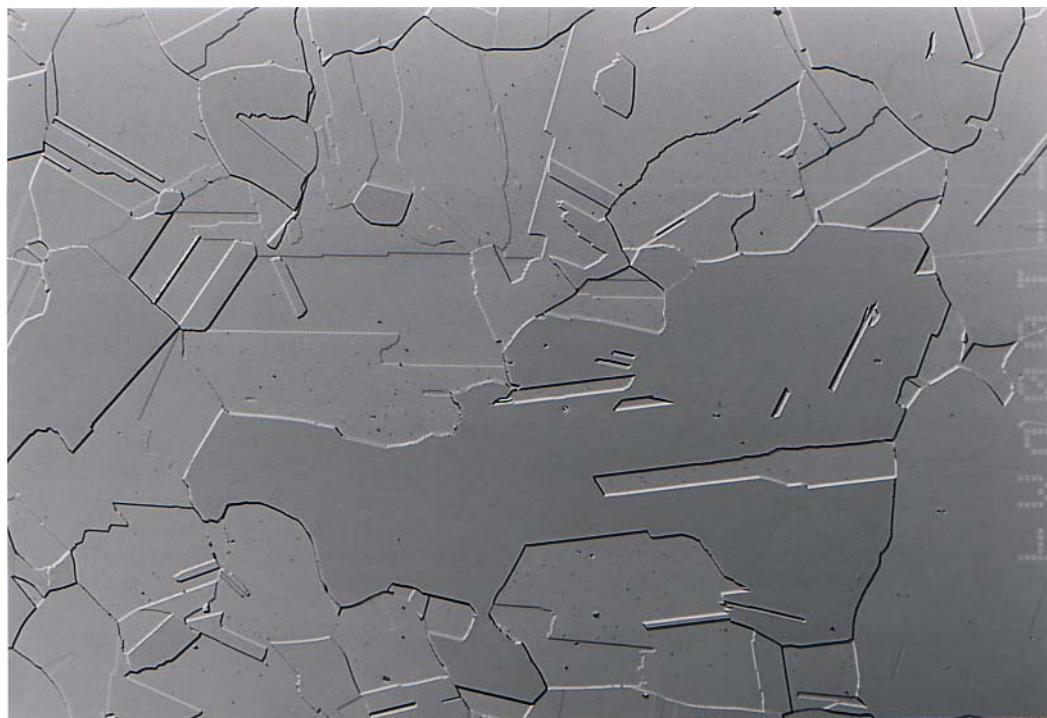
Figure 28: Development of Grain Boundaries and Twins for High-Purity Cu by Ion Beam Etching (Pole pieces, Specimen 4), DIC Micrograph, Section of Figure 27, Parameter: 6 kV / 370 \mu A / 2.4 mins, vertical, rotating
