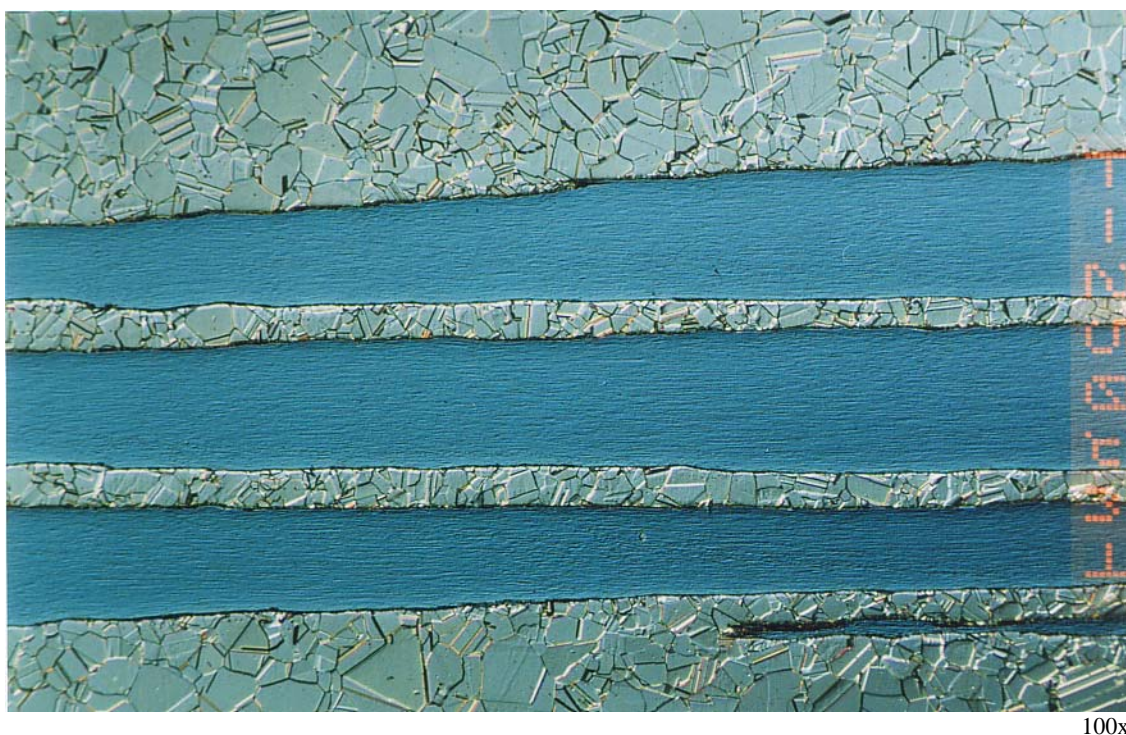
Figure 56: Superconductor CuSn+NbTi+Ta with Cu Layer after Ion Beam Etching (Specimen 2, longitudinal), CuSn Matrix with NbTi fibers, Lower Area of Figure 53, Micrograph with DIC, Parameter: 6 kV / 405 \mu A / 12 mins, 45°, rotating + 6 kV / 405 \mu A / 2.4 mins, vertical, rotating + 6 kV / 390 \mu A / 2 mins, 10°, rotating
