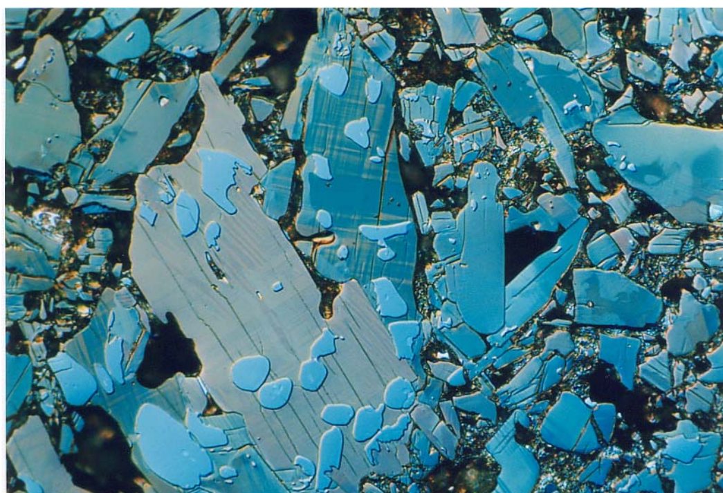
Figure 62: Ceramic Core of the Superconductor with Ag Mantel after Ion Beam Etching (Specimen 1), same position as Figure 61, Micrograph however with Differential Interference Contrast, Parameter: 6 kV / 385 \mu A / 4.4 mins, 45°, rotating
