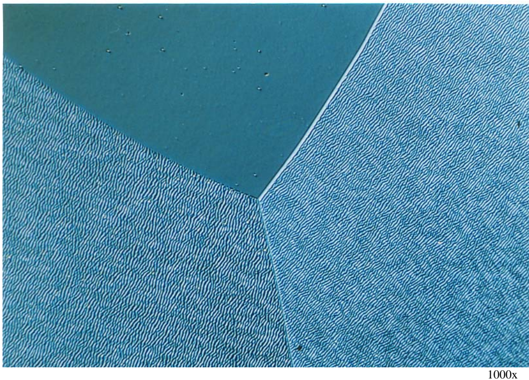
Figure 38: Structure of High-Purity-Aluminium after Ion Beam Etching (Specimen 4), DIC Micrograph, Section of Figure 35 3.1.4.2 Machining Alloy: AlMgSiPb / F28 (Figure 39)
