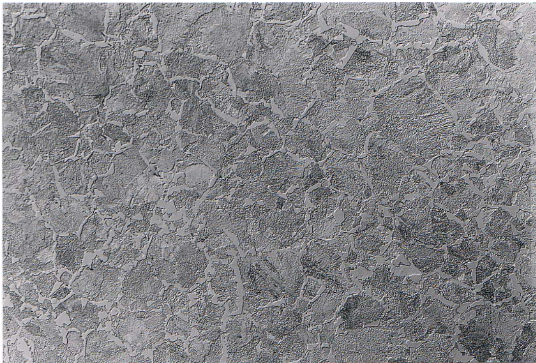
Figure 16: Texture of the Construction Steel Ck45 (Specimen 2.4), Ion Beam Etched, Micrograph Taken between the Etch Points, Parameter: 3 kV / 100 \mu A / 16 mins and 4 kV / 150 \mu A / 8 mins, Perlite developed similarly as when using traditional chemical etch agents
