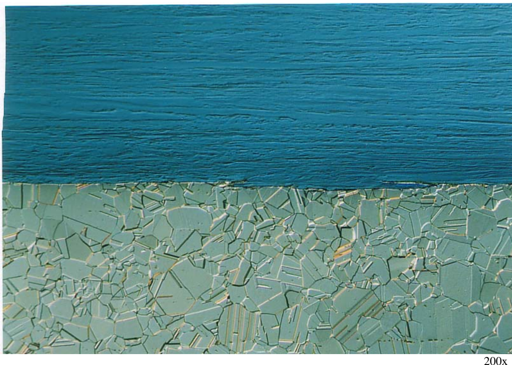
Figure 55: Superconductor CuSn+NbTi+Ta with Cu Layer after Ion Beam Etching (Specimen 2, longitudinal), CuSn with Ta-Coating, Section from Upper Area of Figure 53 Micrograph with DIC, Parameter: multiple etching, cf. Figure 53
