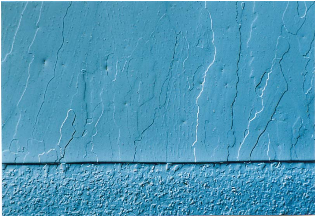
Figure 66: Build-Up Welds derived from a Ni Alloy on Boilerplate HII after Bombardment with Ar Ions (large specimen), Micrograph with DIC, Substrate and Welds Etched, Parameter: 6 kV / 466 \mu A / 8 mins, 45°, rotating + 6 kV / 450 \mu A / 1.2 mins, 45°, rotating
