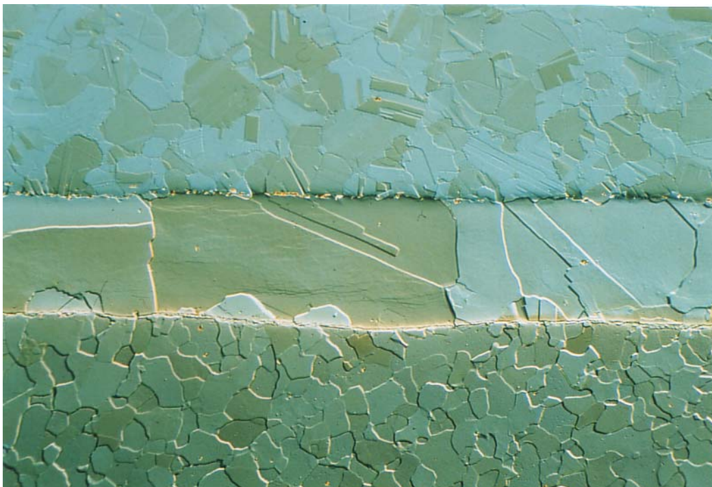
Figure 72: Weld Link of Hastalloy on Plain Steel with Ni Intermediate Layer after Bombardment with Ar Ions and additionally with Oxygen (Specimen 1), Same Position as Figure 71, Enhanced Contrast as a result of Tarnish Layer
