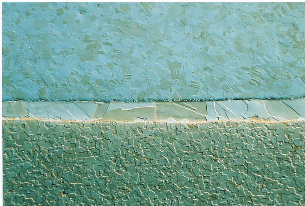
Figure 70: Weld Link of Hastalloy on Plain Steel with Ni Intermediate Layer after Bombardment with Ar Ions and additionally with Oxygen (Specimen 1), Enlarged Section of Figure 69, Enhanced Contrast by means of Tarnish Layer
