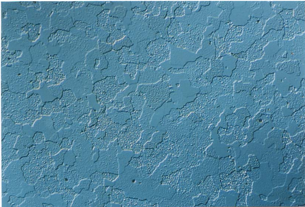
Figure 9: Texture of the Tool Steel 100Cr6 (Specimen 1), Ion Beam Etched, Micrograph from the Edge of the Etch Mark, Parameter: 6.5 kV / 490 \mu A / 8 mins
