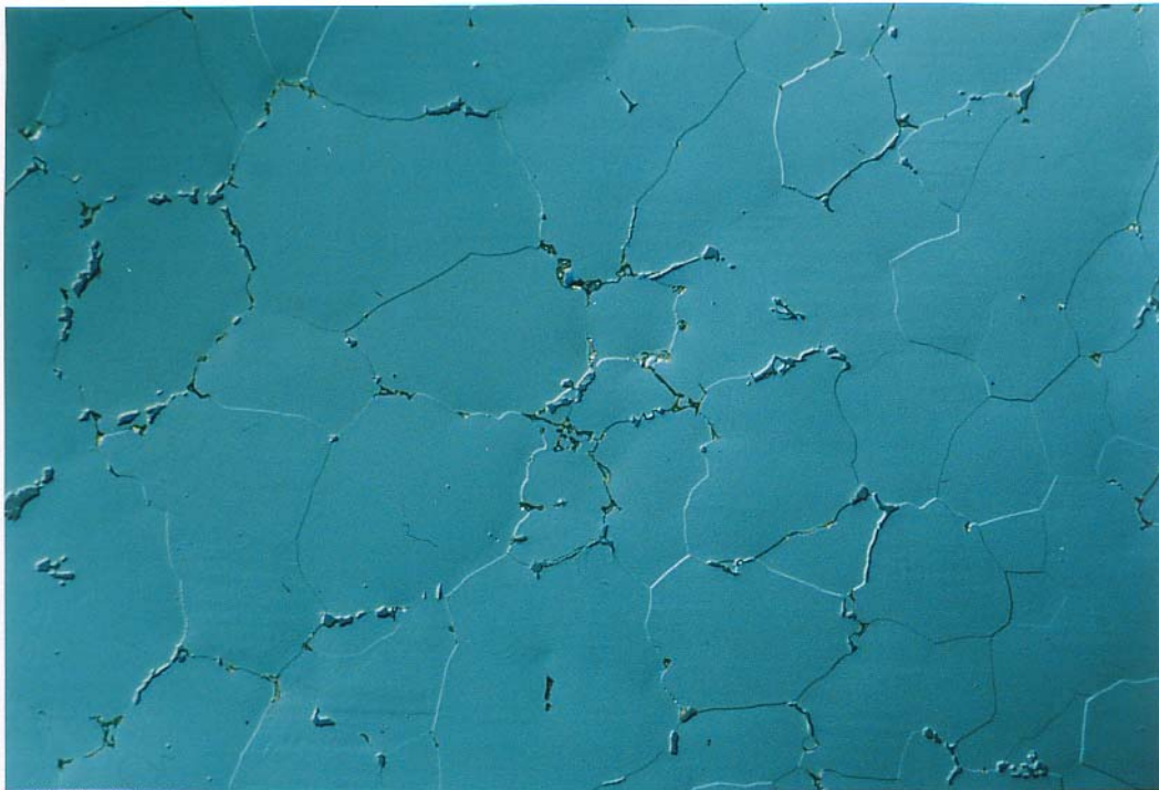
Figure 40: Texture of the Al Casting Alloy AlMg4.5Mn after Ion Beam Etching (Specimen 1), Micrograph with DIC, Grain Boundaries and Intermetallic Combinations Etched,
