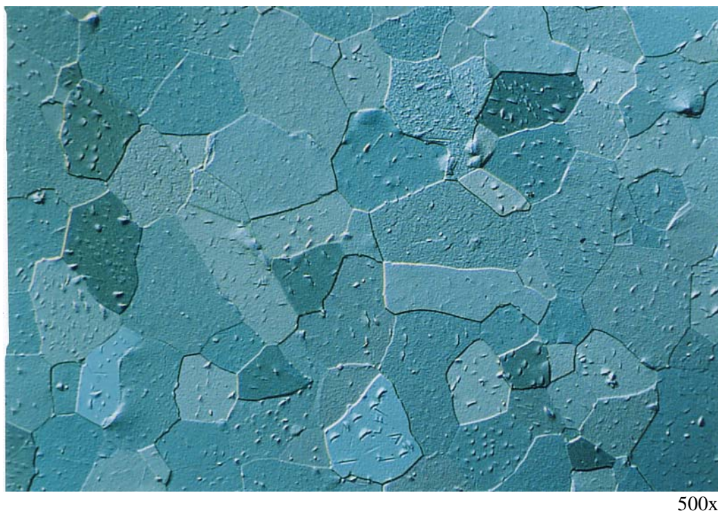
Figure 21: High-Purity Titanium Texture (Specimen 3), Ion Beam Etched, Micrograph with DIC, practically the same position as Figure 20
