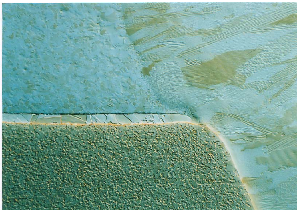
Figure 69: Overview of the Weld Link of Hastalloy on Plain Steel with Ni Intermediate Layer after Bombardment with Ar Ions and additionally with Oxygen
