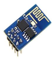
Figure 8: ESP8266 Wi-Fi module
