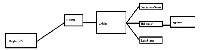
Figure 1: IoT Based Smart Energy Management System
