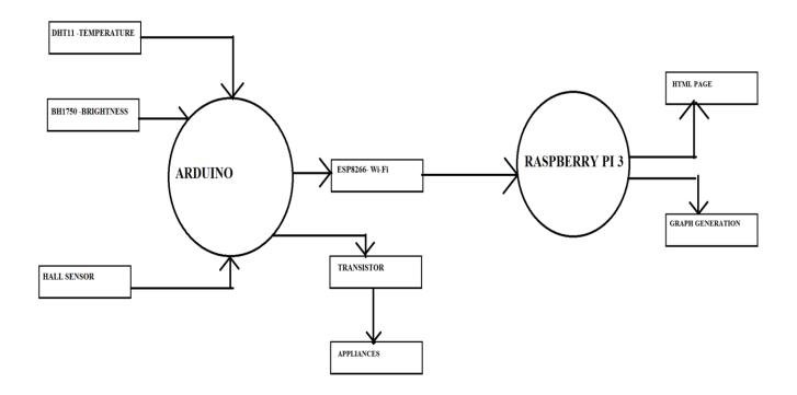
Figure 2: Data Flow Diagram
