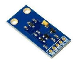
Figure 5: Light intensity sensor
