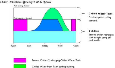
Fig 2 Example utilisation of chilled water storage compared to chiller only approach
