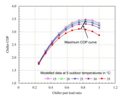
Fig 1 Part load performance curves of a chiller operating under head pressure control. (source: Yu & Chan)<sup>2</sup>
