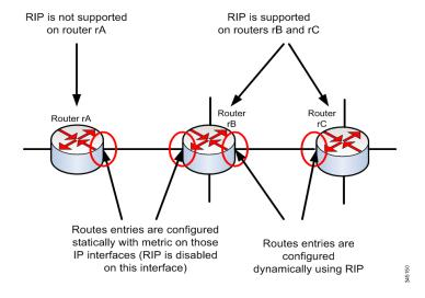
Router rA does not support RIP. Therefore, routing entries with an appropriate metric are configured statically on this router. While on router rB the route to router rA is considered a connected route. In contrast, routers rB and rC derive and distribute their routing entries using RIP.
