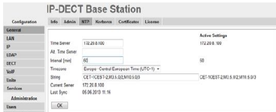
Figure 4. Configure NTP settings
