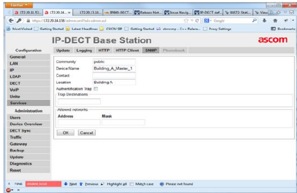
Figure 7. Configure SNMP Settings
