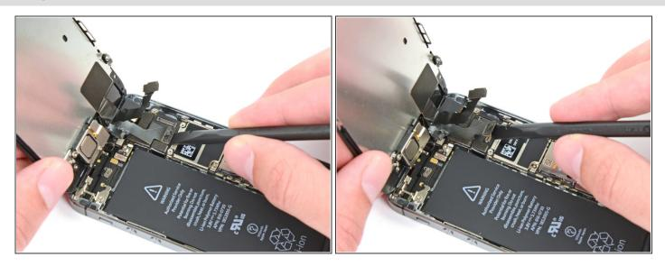
• While still supporting the front panel, disconnect the digitizer cable connector.
