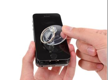
Do not try to completely remove the front panel assembly from the rear case, as there are several ribbon cables still attached at the top of the iPhone.
