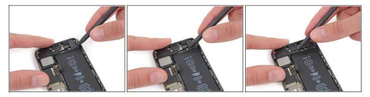
Run the tip of a spudger between the battery and the headphone jack to unfold the battery adhesive tab.
