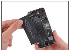
Pull the battery out of the rear case.
