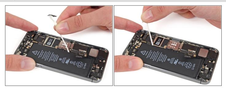
• Pull the strip along the side of the battery until the strip comes free from the phone.
