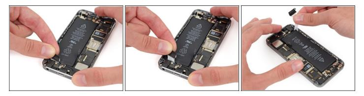
Pull the outside battery adhesive tab straight up and carefully around the corner of the battery.
