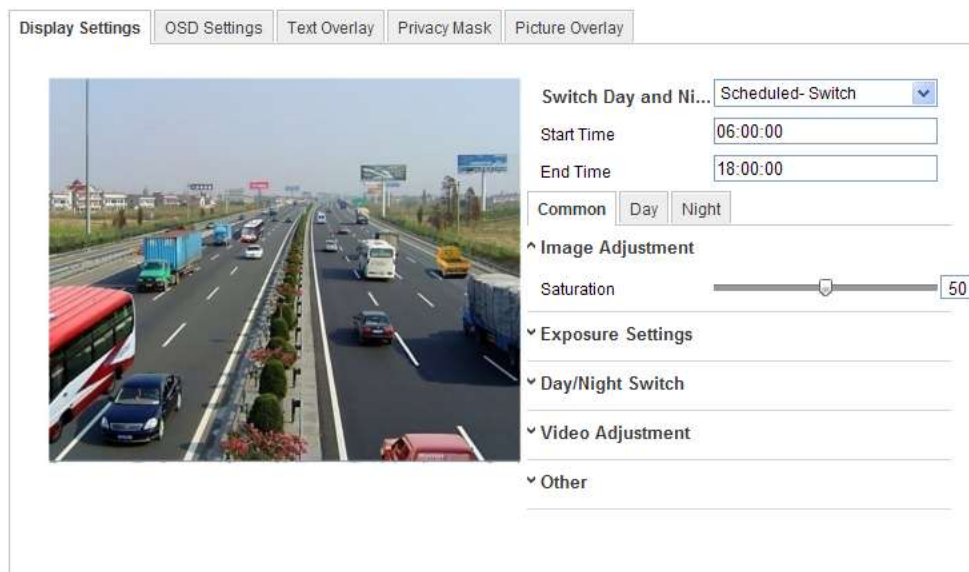
Figure 6-33 Day/Night Scheduled-Switch Configuration Interface
