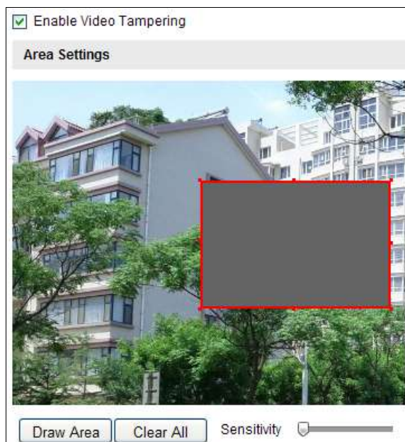
Figure 6-47 Video Tampering Alarm
