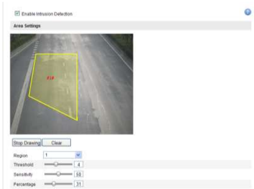
Figure 6-55 Configuring Intrusion Area
