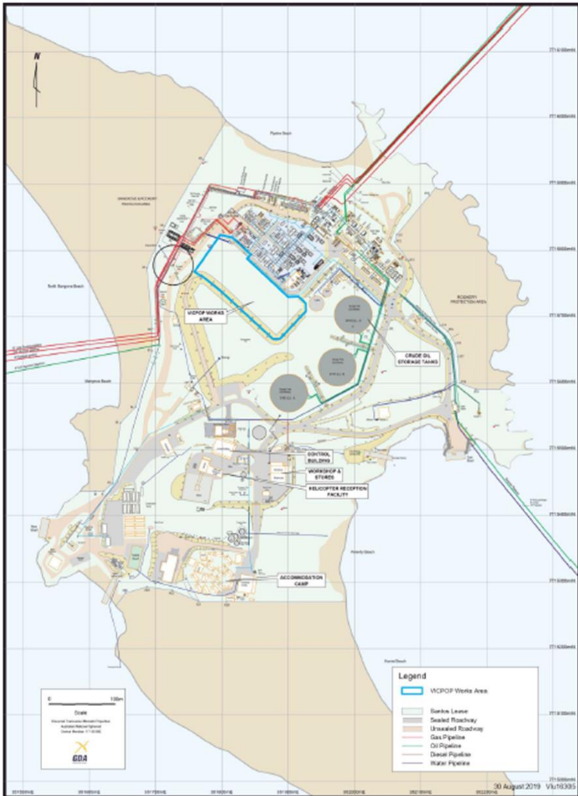
Figure 3: The layout of the Santos WA Energy Limited Lease area and the existing Varanus Island infrastructure
