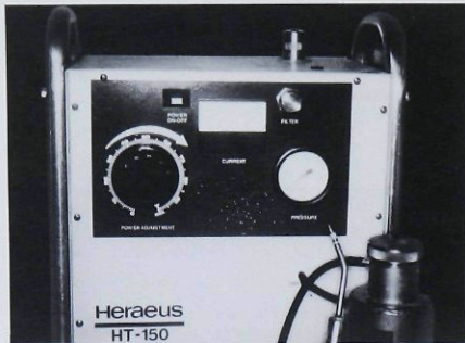
Fig 6 Hydrolysis machine (source of hydrogen and oxygen gases).
