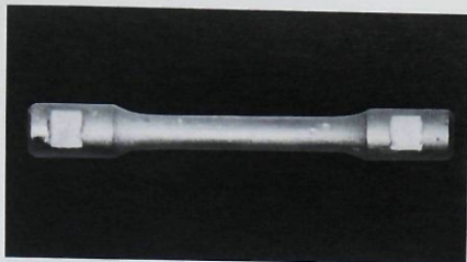
Fig 2 Specimen cast in palladium-silver alloy.
