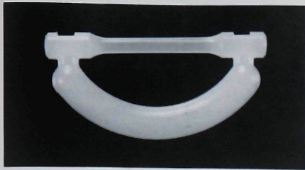
Fig 1 Prefabricated wax pattern for tensile test rod.
