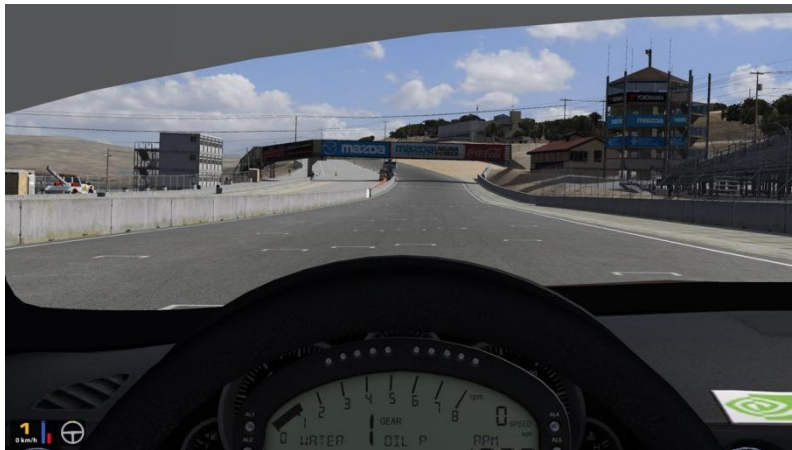
A field of view of 45° cuts off important information from the focus area, but increases object size.
